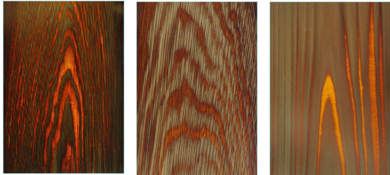
Densified wood veneers illuminated from the back (from left: oak, oak, beech)
